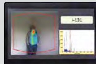
Display of dose rate on LCD screen on RAVIN CAM. Imaging of activity during patient release survey after 131 I radio-ablation.
