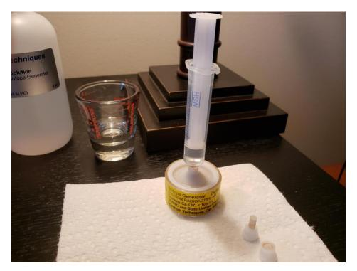
Now, place <u>4 drops</u> of the barium solution into the planchet from above. Try to center the drops in the planchet.
