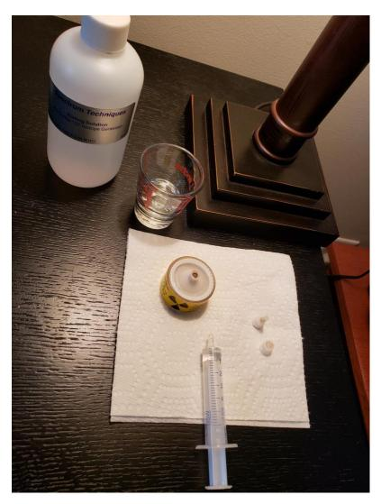
Attach the syringe to the CORRECT side port of the generator. This is the slightly larger opening – note that there is a FLOW direction arrow on the GENERATOR. The arrow IS NOT pictured here.
