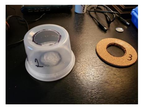
Now put the PART 3 (cork board) below the PART 1/2 assembly and press in. This flattens PART2 and adds stability to the jig. This is your "jig base." Set this aside.
