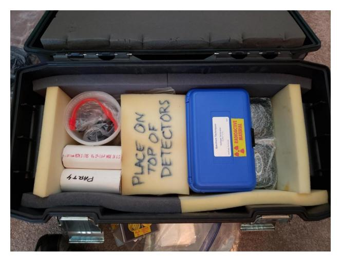
Remove the piece of detector probe padding and the Cs/Ba generator. You should now see the picture on the next page:
