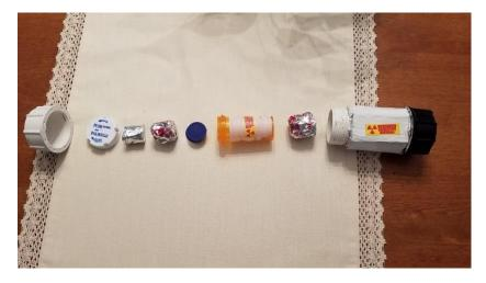
Disassemble down to the source sleeve and remove button sources for use. Re-assemble in reverse order when you are done.
