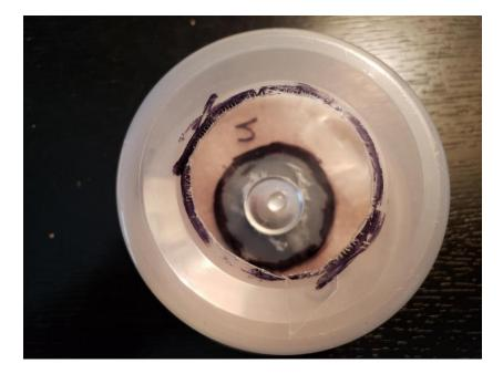
Insert the probe assembly into the jig base and slowly position the bottom end over the planchet until the sleeve touches the jig base.
