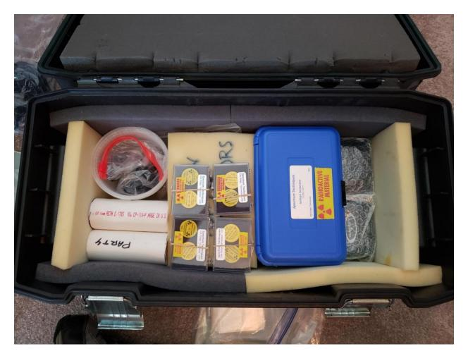
Parts 1 and 4 for the detector Jig are to the left. A bag of large paper clips used for mounting the button sources are inside the stack of 4 Jig Part 1's. The Vernier Interfaces are below the Cs/Ba generator. Remove the 4 plastic boxes containing the Co/Sr sources. You should now see this on the next page:
