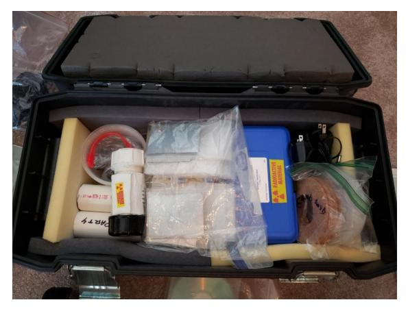
Remove the lab experiment shielding pieces (in bags) in the center. Two Vernier power supplies are top right. Remove the Jig Parts (2 and 3) for mounting the radiation detector are at (bottom right). The Cs/Ba generator is the blue item under the shield packets. The Cs-137 source storage tube is to the left (it has a white cap and black cap). You should now see the picture on the next page:
