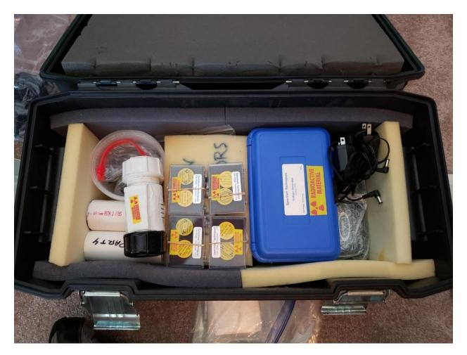
Parts 1 and 4 for the detector Jig are to the left. The source storage tube, 4 sets of Co-60, Sr-90 button sources are next followed by the Cs/Ba generator. Remove the source storage tube and the two Vernier Interface power supplies. You should now see the picture on the next page:
