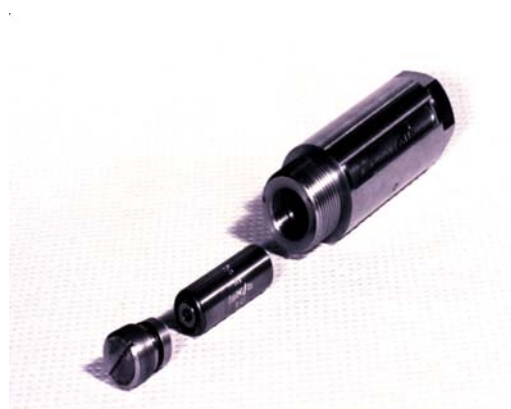
Figure 2.5 Well-Logging Source and its Pressure Vessel
