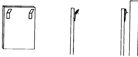
Figure 6. A method of invisibly attaching poster components to display board.
